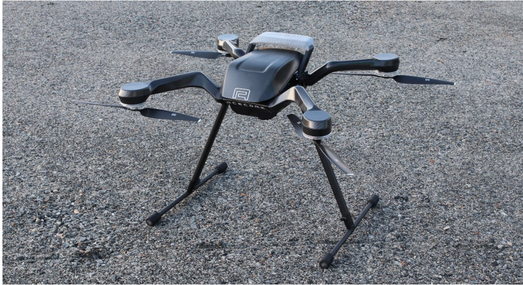
Figure 5 Acecore Zoe, the quadcopter used as a basis for the presented drone system
